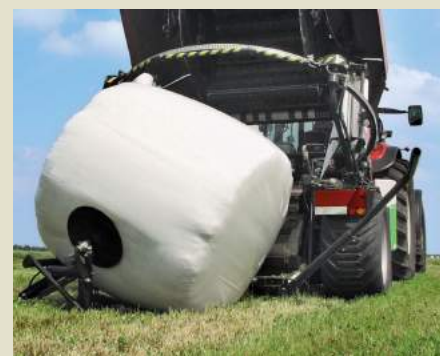
Bale turner, unloading the bale on its flat end
