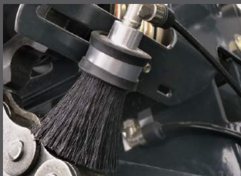
Standard Beka Max chain oiling system
